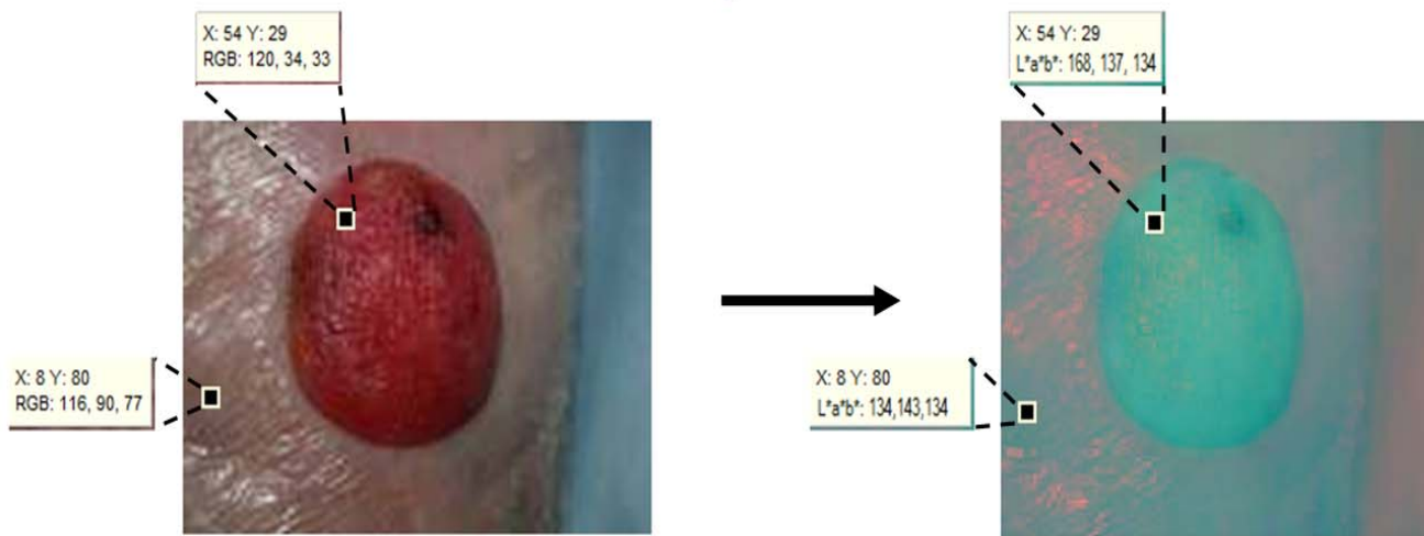
Fig. 1. Conversion of Lesion Image from RGB colour space to CIE L*a*b* colour space showing the corresponding pixel values for different pixels of the same image in two different colour spaces.
